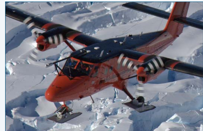
▲ A BAS Twin Otter aircraft fitted with a meteorological probe for air sampling
